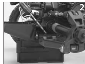
Keep the drill bit perpendicular to the flat surface of the hole location. (Wheels removed for printed instruction purposes only, the procedure can be performed with wheels in place)
