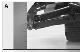
As the down travel is adjusted, measure the distance from the lower outer edge of each suspension arm to the surface.
