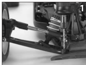
Keep the drill bit perpendicular to the flat surface of the hole location. (Wheels removed for printed instruction purposes only, the procedure can be performed with wheels in place)
