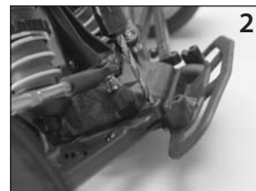
Keep the drill bit perpendicular to the flat surface of the hole location. (Wheels removed for printed instruction purposes only, the procedure can be performed with wheels in place)
